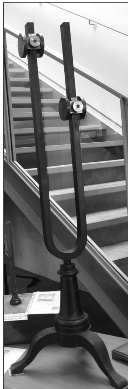
Fig. 1 Very large tuning fork by Rudolph Koenig with adjustable frequency (16 to 24 Hz).
