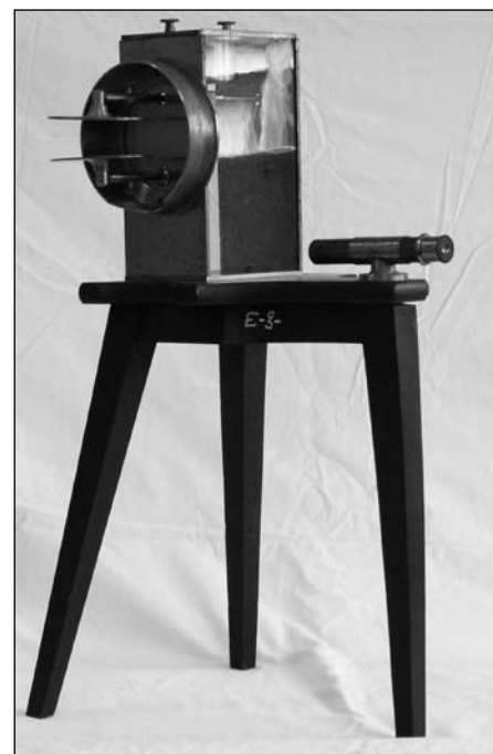
Fig. 5 Pierre Curie's gold-leaf electroscope.
